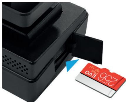
**CAUTION!** Attempting to insert a memory card wrong may damage the device and/or the memory card itself. Make sure the memory card is in the correct position. Do not apply excessive force when inserting a memory card.
