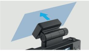
**CAUTION!** Adjusting the viewing angle can only be done along the vertical line, so be sure to position the device correctly on the windshield along the horizontal line as close as possible to the windshield's center.
